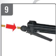
**Attach spray tube to trigger valve and tighten**
