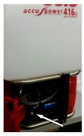
2. Locate the positive battery lead (red wire) remove the insulation, either a yellow type as shown below, or a black heat shrink tubing will be found on some units covering the blade connector.
