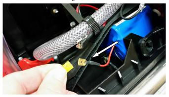
3. Securely insert the blade connector into the plug as shown below.
