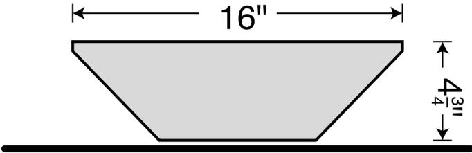
The Junior™, mounts like the rest of the 601 series of traps, in a corner or flat against the wall.
