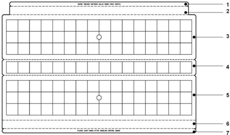
**Genus<sup>®</sup> Spectra:** Two halves of the complete universal control board are used. Tear off and discard section 4. Use one half of each board in the upper and lower sections.
