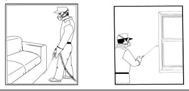
**Helpful Hints:** Occasionally, when working overhead, the pressure exerted on the liquid tank by the regulator will not be sufficient to drive the liquid 8-10 feet above floor level. At this time, you need to increase the pressure on the liquid tank by adjusting the regulator clockwise to the point you receive the aerosol at the tip and at the height you desire to work.
