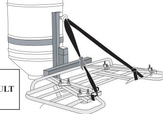
FAILURE TO PROPERLY CONNECT AND MONITOR THE RATCHET STRAP MAY RESULT IN DAMAGE TO THE ATV OR SPREADER
