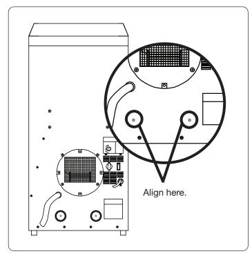
**Step 2:** Attach the condensate pump using the two screws as shown. Do not over tighten the screws.
