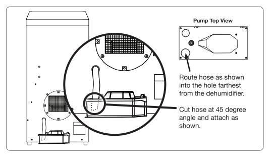
**Step 4:** Insert clamp onto 3/8" drain hose and then attach hose onto the barbed outlet fitting on the condensate pump. Tighten clamp and verify that hose is secured tightly to the condensate pump by gently pulling on the hose. Route hose appropriately to drain.
