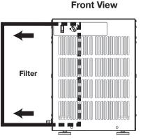
**Step 3** - Insert the new filter into the filter compartment and attach the magnetized filter door back into place, ensuring it covers the filter compartment completely. Be sure the arrows on the filter are facing into the dehumidifier.
