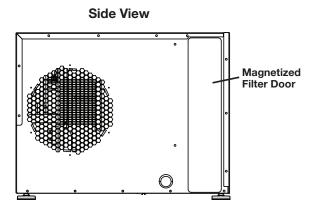
**Step 2** - Remove the filter by pulling it out of the filter compartment.
