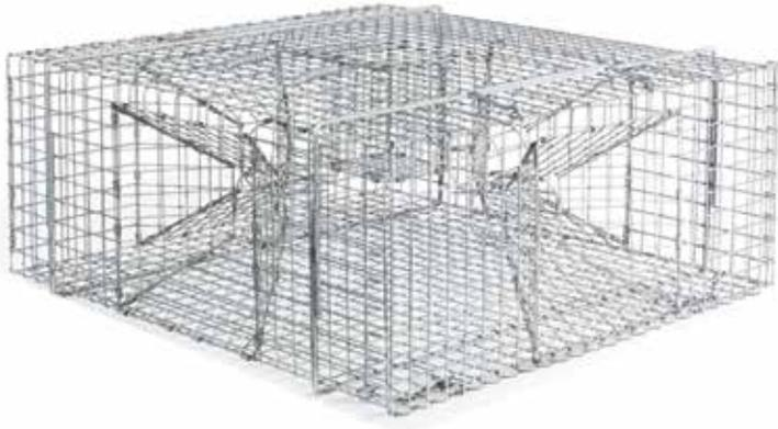
**Model 405.5 – Repeating Crayfish, Crab, and Shrimp Trap** featuring three funnel style trap doors. This heavy duty trap measures 24W x 24L x 9H and is constructed from 1 x 1 – 14 gauge galvanized wire mesh. It includes a 4 x 4” built in bait box constructed from ½ x ½ galvanized wire mesh. One entire side of the trap can be quickly unlatched and opened to allow for easy unloading of your catch.
