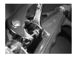
The check valve, at the base of the pump cylinder, can be removed and cleaned, and the base of the cylinder (around the holes) should be cleaned of residue. Tightly replace the check valve, and be certain it is secure.
