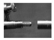
A 3/8 open-end wrench can be used to tighten the packing nut if the valve develops a leak.
