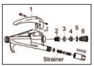
Remove the Trigger (1), then the Snap ring (5), Safety lock nut (6), the Adjustment screw (4), the Lock nut (3), and then the Packing nut (2). The Trigger can be removed by moving it to the back of the Valve.
