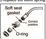
**Problem:** Hose is leaking at the connection with the tank; leaks when tank is pressurized.
