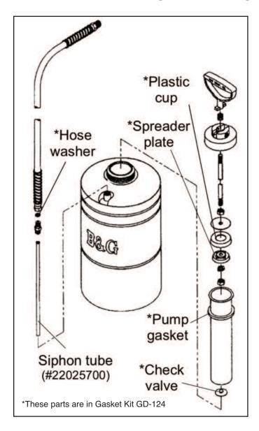
**Problem:** Tank is not holding pressure; pump is working but no pressure remains in the tank.
