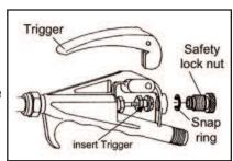
Attach the tip and nozzle to the end of the Extension, make certain the Soft seat gasket is facing correctly. The small end faces the Extension. Press the Trigger to retract the Seat stem into the Extension, then attach the tip and nozzle.
