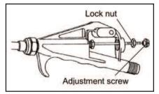
the top of the slot in the top of the screw. Tighten the Lock nut against the screw.
