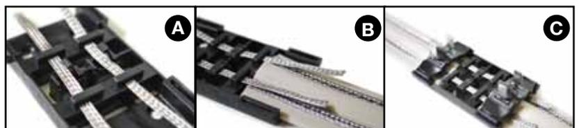
side, take the track and place in the remaining trough, put the braid down on top and press the cap down until it locks. (D & E) To make sure you don't have any short circuit, trim off all excess pieces of braid. (E) Notice that the two male connections sticking up can be used to connect to a lead wire or another track. If not being used, make sure you bend them down away from each other to prevent arcing.
