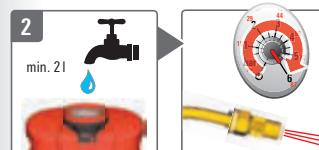
**Fill up with clean water, switch on sprayer, set adjustable nozzle to jet and spray until no more liquid comes out**
