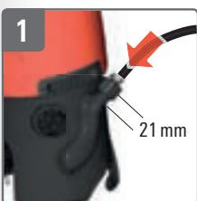
Screw hose onto air chamber
