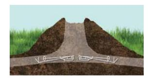
**STEP 5:** Place the traps in opposite directions (2 traps are recommended for the best results). It is not necessary to cover the opening unless you are concerned with pets or other interference. When the mole or gopher returns to investigate the disturbed tunnel area, it will activate the trigger and the powerful spring steel jaws will close around the middle of its body causing instant results. Remove the trap, replace the dirt and continue to observe the area for further activity.
