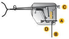
**STEP 3:** Position the rear set wire B across set wire A. Push the trigger wire C forward making sure the set wire B is positioned behind the tab as illustrated. When you push the trigger wire C you are in the guide area on the rear of the trap base.
