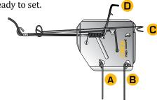
**STEP 2:** Holding the trap firm with one hand, raise the active jaw wire D and lower it to the opposite side of the trap base. Position the forward set wire A across the active jaw wire D as shown.
