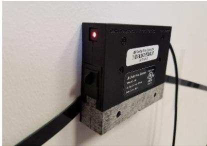
**STEP 2:** If the device is alerted, ensure both doors are fully closed prior to removal for visual inspection.
