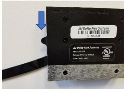
**STEP 3:** Grab the tab on the chamber door and pull the chamber out of the device as shown below. *The door must be closed for chamber removal.*
