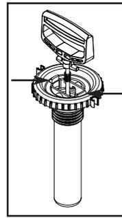
To dislodge pump barrel from cap, push the 2 ears forward and down through the cap. Make sure pump cup is well greased.
