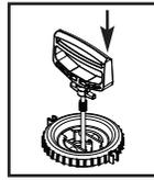
To lock handle, push handle down, to depress coil spring and turn handle 1/4 turn clockwise then allow handle to rise into lock position.
