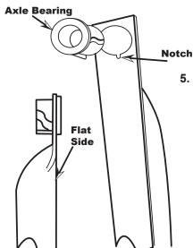
**5.** Install the bearings over the axle and press into the notches of the lower handle as shown above.
