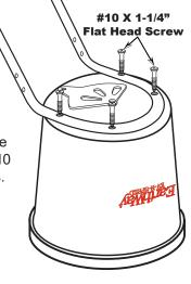
3. Install gear box by inserting the pinion shaft into hole in center of hoppers bottom. The ARROW on the gearbox must point to FRONT of the hopper. Follow label instructions on hopper.
