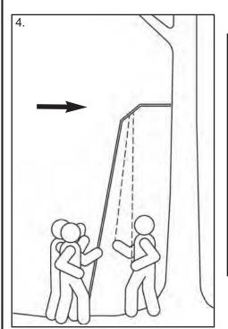
4. As tree stand is being raised, the person holding Installation Straps will pull toward themself to take up slack. It will steady and ease the weight of stand on the other two people. Continue walking stand upward, until Tree Contact is resting against the tree.
