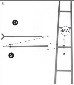
5. Slide the inner part of the Stabilizer Bar into the outer part. Attach Stabilizer Bar ① to the bracket attached to the second rung of the Middle Ladder Section with 1 - 45W bolt and 1 wingnut.
