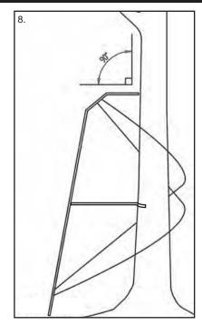
8. Cross Installation Straps behind tree. Attach to the bottom ladder section by following **Installation Strap Instructions Page 2.**
