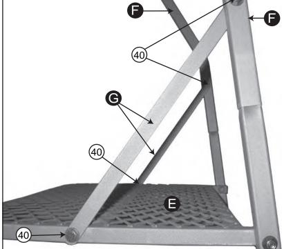
8. Attach one end of the Platform Support **G** to Foot Platform **E** using **1 - M12x40mm bolt** for each side. Attach the other end of Platform Support **G** to the inside of Handle Rail **F** using **1 - M12x40mm bolt** on each side.
