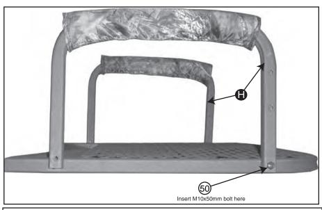
2. Attach Arm Rest Cover M to each Arm Rest H . Attach the front of Arm Rest H to Seat Platform D using **1** - **M10x50mm bolt** on each side.
