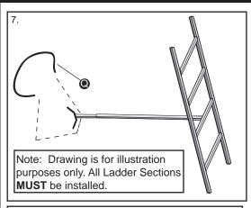
7. Tie one end of Tiedown Rope (a) to the inner part of Stabilizer Bar near the flanged end. Wrap the rope around the back of the tree once. Then tie the other end of the rope to the stabilizer bar.
