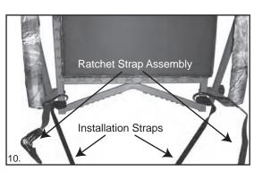
10. Attach one end of Ratchet Strap **(R)** to one side of the rear of the seat platform. Wrap strap around the back of the tree once and hook to the other side of the rear of the seat platform **(See Ratchet Strap Instructions)**. Ratchet strap tight.
