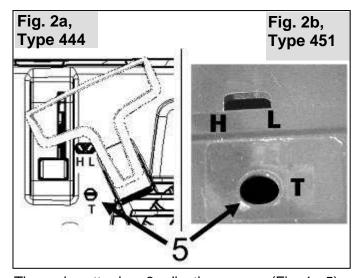
The carburettor has 3 adjusting screws (Fig. 1 - 5):
