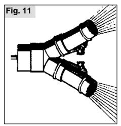
Remove standard nozzle (4) from the spray wand and push the dual nozzle onto the spray wand.
