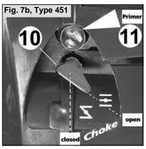
Close choke with choke lever (10).
