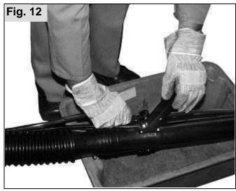
Above the container, pull the supply hose from the shut-off valve.
