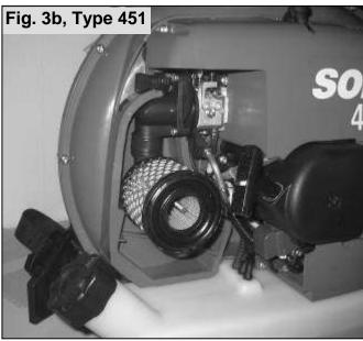
Undo the screw (Fig. 1, Pos 8) completely (screw is retained inside the filter cover) and remove the filter cover.
