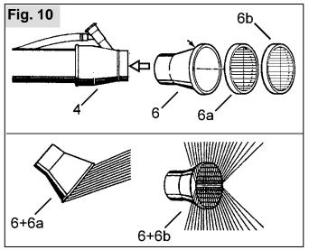
The nozzle attachment (6) is positioned onto the standard nozzle (4) with the selected grille.
