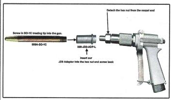
With the JD9 Adaptor, the PMP can convert the Pro-Pest®505 Spray Gun or JD9 gun into a termite treating tool. It's as easy as 1,2,3! Simply detach the hex nut from the nozzle end, insert our adaptor into the hex nut and screw back into the gun. Screw in the treating tip (SO-1C) and it's ready to go!
