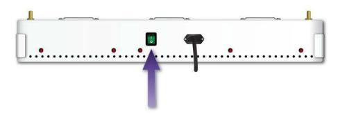
There are certain diodes that emit Infrared light and others emit UV light. The IR diodes appear to be off and the UV diodes emit a dull blue light. Do not be alarmed as these diodes are on, working properly, and doing their job.
