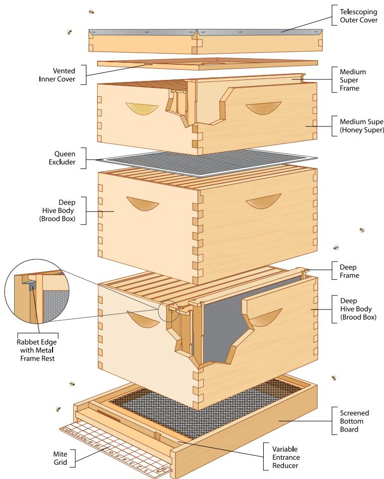
**Queen Excluder** (*QEPL sold separately*) A flat plastic sheet with holes large enough to allow the worker bees through but small enough to keep the queen from moving upward in the hive. It is to be placed between the highest brood box and the first honey super, preventing the queen from laying eggs in the place where the honey is to be harvested.
