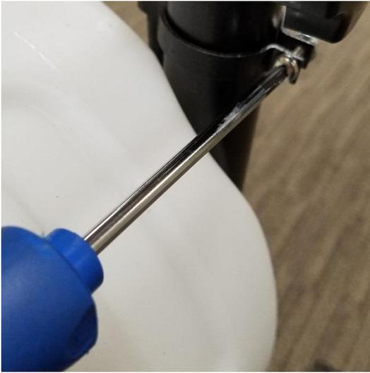
Secure the Wire Clamps on the Handle and Lower Frame using the Phillips Screwdriver.
