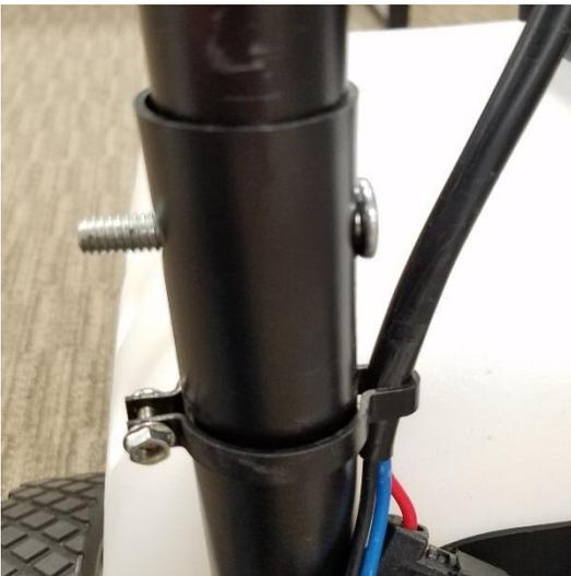
Adjust the Handle to a comfortable height for the operator, and find the hole nearest this position that aligns with the hole in the Lower Frame. Insert the Handle Adjustment Bolts (from kit 33-100157) through the holes.
