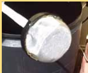
Suction filter after Naprovit fill
