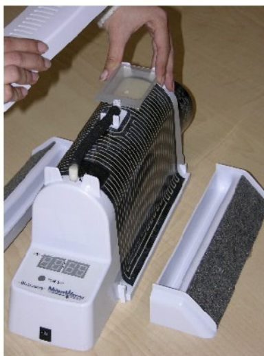
Figure 5 Attach kairomone lure and vented cover
