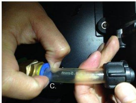
Once the blue ring is against the brass fitting, the tubing pulls right out. (below)
