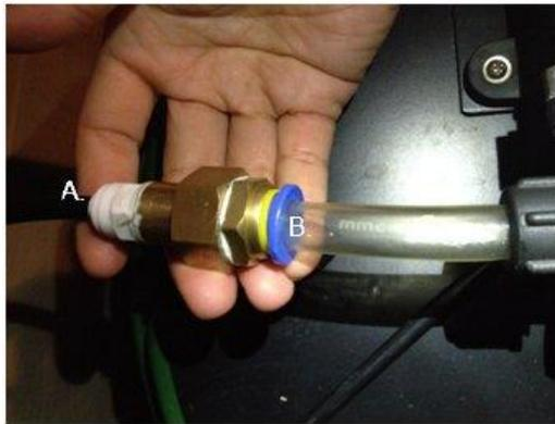
DO NOT ATTEMPT TO REMOVE TUBE FROM POINT “A”. **Once you have inserted the tubing in “A”, it cannot be removed.** However, you may remove the tubing from point B. (Above)
