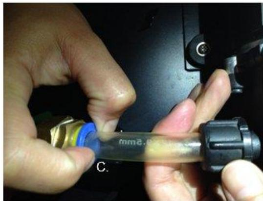
Once the blue ring is against the brass fitting, the tubing pulls right out. (below)
