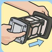
**5.** Remove the butane cartridge cap. Screw the cartridge into the center of the lantern globe. Make sure the cartridge is fully inserted by turning it clockwise until it stops. Replace lantern globe on base. One ThermaCELL® butane cartridge lasts a maximum of 12 hours.
