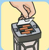
**2.** Remove one ThermaCELL® mat from wrapper. Mats last a maximum of 4 hours. Mat turns from pale blue to white when repellent has been exhausted.
