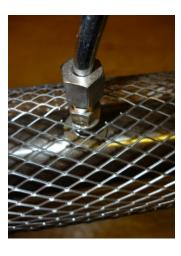
• Check there is no leaks in the chemical tank. Blow compressed air backwards though the chemical tube from the inlet nozzle to see if any bubbles appear. Replace leaking parts if necessary.
