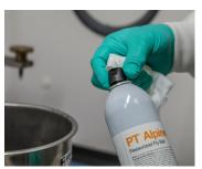
4. Shake the can and turn it upside down. Press the nozzle until spray comes out.
