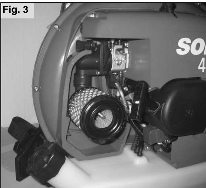
Undo the screw (Fig. 1, Pos 8) completely (screw is retained inside the filter cover) and remove the filter cover.
