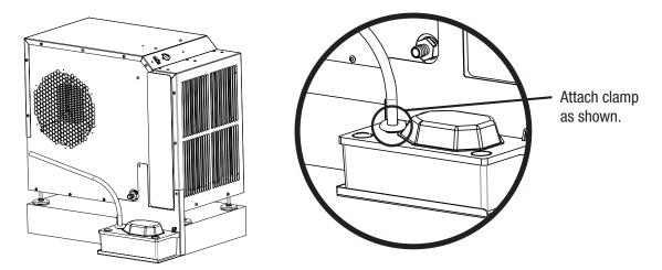
**Step 6:** Attach 5/8" hose onto the barbed drain adaptor of the dehumidifier. Route hose to condensate pump as shown. Insert hose no more than 2" into condensate pump. It may be necessary to trim hose to properly fit.
