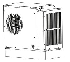
**Step 2:** Knock inlet hole out of the condensate pump in the location shown. ( )
