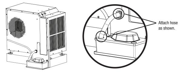
Step 7: Plug the pump and dehumidifier cords into an outlet that is protected with A GFCI device on its circuit.
