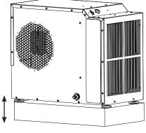
**Step 3:** Using a T25 Torx driver, remove two screws located on the side of the unit as shown.
