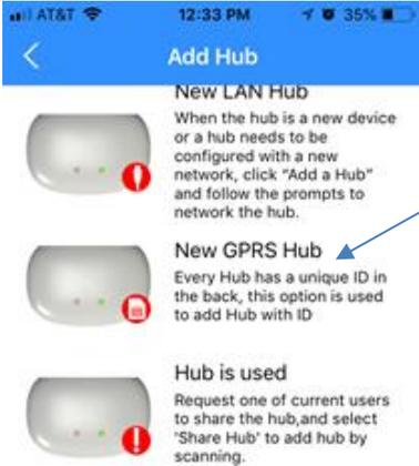
You can add the hub by either scan the QR code, or, select "New GPRS Hub" then type in the serial number below QR code.
