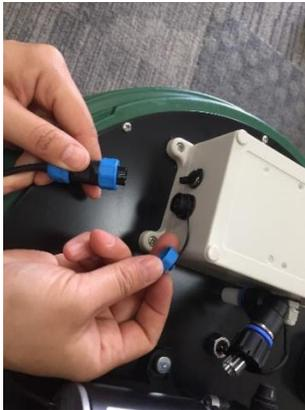
Plug the power cable onto the controller. Screw in the blue connecting nut.
