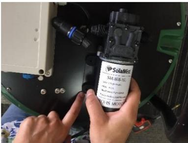
To install pump, you will need to secure the four rubber feet into the main unit first by using the included bolts.
