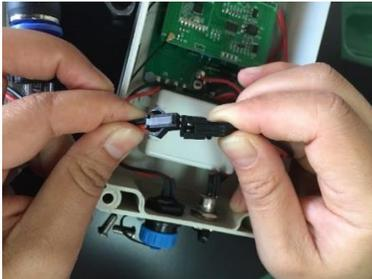
The male and female plug of the battery has to be connected correctly. Check all connections to make sure they are all secure. Screw the cover back on the base and replace the scrow hole plugs.
