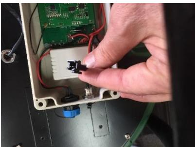
Inspect the the plug for the battery to make sure the two metal prongs are in good shape.
