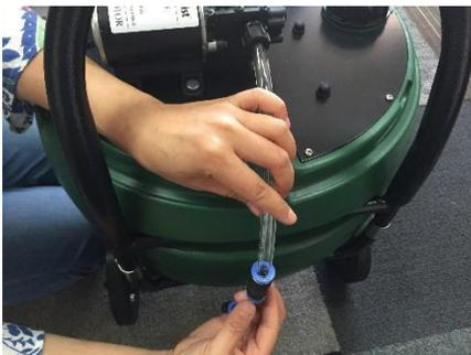
Connect the pressure regulating tube, the small black tube included in the pump assembly.
