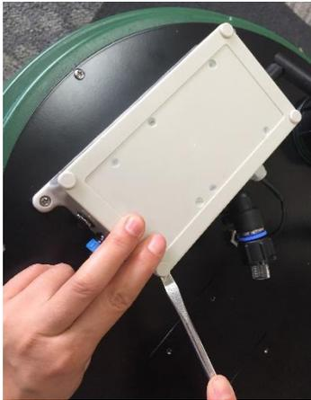
Battery is included but NOT preinstalled. To install battery, gently pry open the plugs on four corner to reach the screws that secure the top part of the controller to the base.
