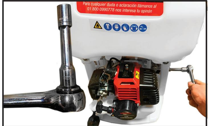
**2** Using a 10mm socket wrench, loosen the 4 bolts on the right & left sides of the pump.
