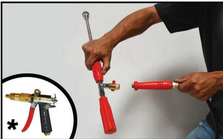
**3** Fasten the sprayer attachment to the valved end of the hose.
