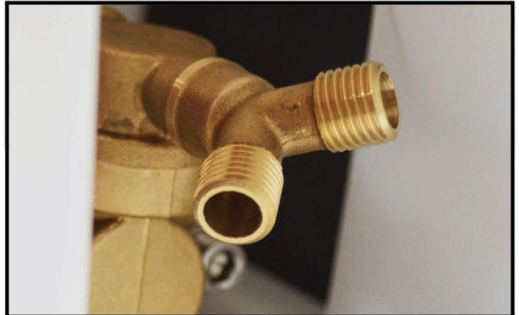
**4** Fasten the Y connection fitting clockwise around the opening of the pump, until secure.
