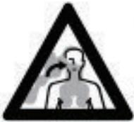
Toxic exhaust fumes may be colorless and odorless and contain unburned hydrocarbons and benzol. Never operate the power tool in enclosed or poorly ventilated locations.
