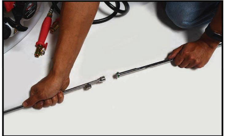
**8** Fasten the bottom end of each wand to the top (curved) end.
