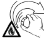
After fueling, tighten down the screw-type fuel cap as tight as possible.
