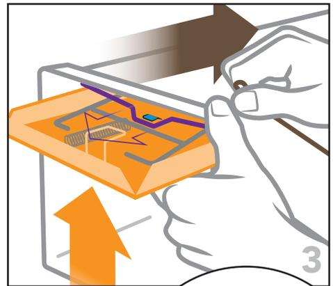
1. Locate and lift the **(A)** door lock latch, the small wire located at the top, front, center of trap. See above. Lift portion of latch nearest the front of the trap so the latch inside the trap is flush against the top inside of the trap. This will allow the door to move freely.
