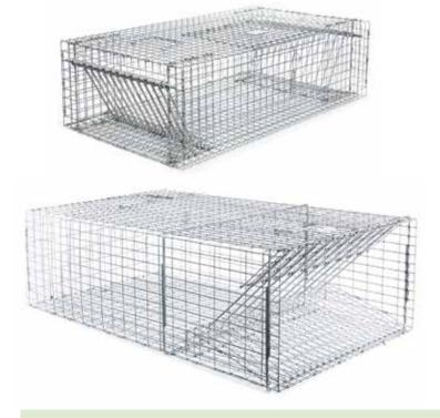
**Model 450 – Repeating Turtle / Reptile Trap** designed to catch and hold multiple turtles at a time. It measures  $32L \times 18W \times 9H$  and features two,  $14W \times 7H$ , repeating trap doors. The doors are made of 6 gauge metal bobs that swing freely inward to let animals enter but cannot be pushed open from the inside. Trap also features an easy bait and release door on the top of the trap. Trap frame is constructed from  $1 \times 1 - 12$  gauge galvanized wire mesh.
