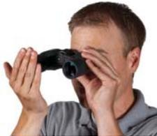
**2. Adjust the diopter**—start by closing your left eye or covering the left objective lens with your hand. Look through your right eye and adjust the diopter ring (found on the right eyepiece) until the object is in focus. Make note of this diopter setting in case you need to set it again. From this point on, you will only need to use the center focus wheel.
