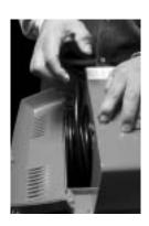
When transporting the machine, make sure the hose is not attached.
