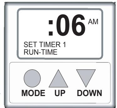
**SET RUN DURATION:** Press the MODE button again to set the RUN-TIME SECONDS which can range from zero to twenty seconds. Adjust RUN-TIME SECONDS using the chart below. Set the RUN-TIME SECONDS to zero to disable the specific timer.
