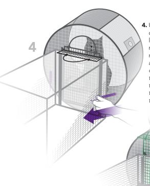
4. Use the extra spring clips located to the left and right of the release door on the roundhouse trap to attach your cage. Be careful not to attach the spring clips so tight that you cannot open the release doors of the trap and cage.
