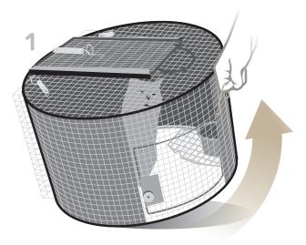
1. Move the trap in the upright position by taking hold of the square handle located on the side of the trap and lift up. Set the trap down on the trap foot which is attached to the side opposite the square handle.
