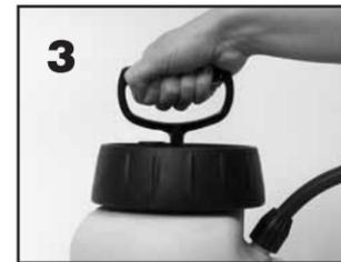
**3** Push handle, down, turn 1/4 turn clockwise to lock. Begin spraying. Re-pump sprayer as required to maintain spray force.
