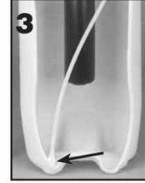
**3** Proper placement of white outlet tube.
