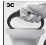
3C **Do:** Push handle, down, turn 1/4 turn clockwise to lock. Begin spraying. Re-pump sprayer as required to maintain spray force.
