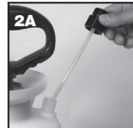
2A Insert tube into tank.
