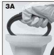
3A **Do:** Turn handle clockwise to tighten. Push handle down, turn 1/4 turn counterclockwise to release.
