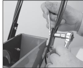
Using 4 nuts and 4 bolts, secure handle bar to hopper/wheel assembly as shown
