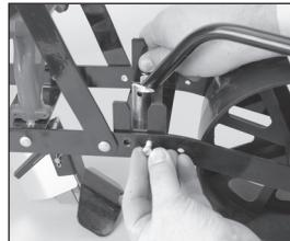
Align base plate of row marker with the 4 corresponding holes on the hopper/wheel assembly as shown.
