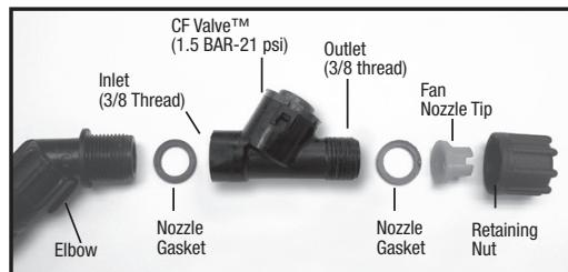
The CF Valve™ is intended to be used with a fixed nozzle. The Fan nozzle tip provided is rated @ .4 GPM @ 40psi.
