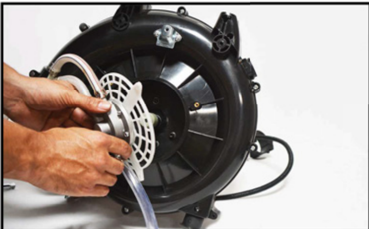
23 Fit the booster pump onto the plastic coupling
