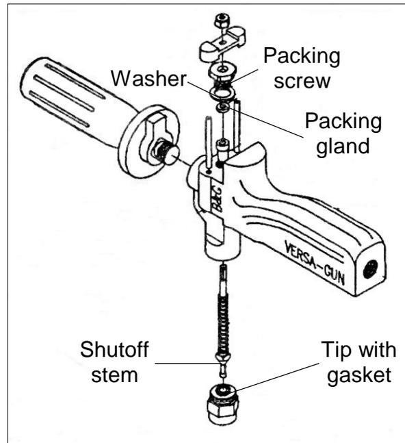
**P.** Leaking occurs at the back of the Valve.
